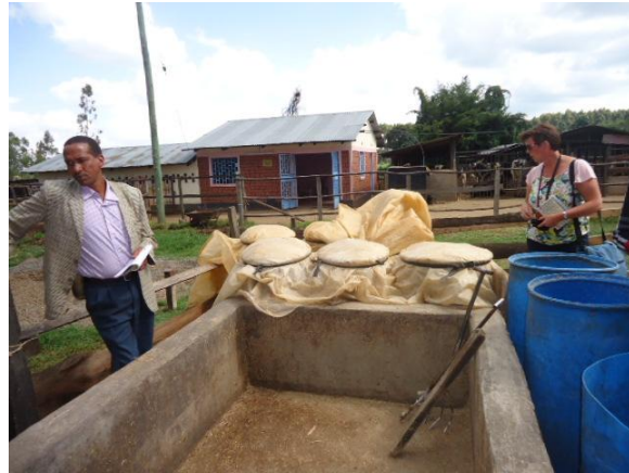
Dairy Feed Mixing Tunnel and Fermentation Tanks, Wilsam Dairies.
